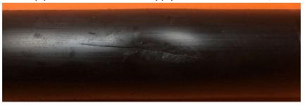
Howard said that the  $\frac{3}{4}$ " plastic pipe is rated for 150 psi compared to 250 psi for the 1" plastic pipe that is used for most of the water feeder pipes to the condos. I measured the wall thickness of the  $\frac{3}{4}$ " plastic pipe at 0.135" compared to 0.176" for the 1" plastic pipe. The wall thickness of the 1" pipe is about 30% greater than the  $\frac{3}{4}$ " pipe.
