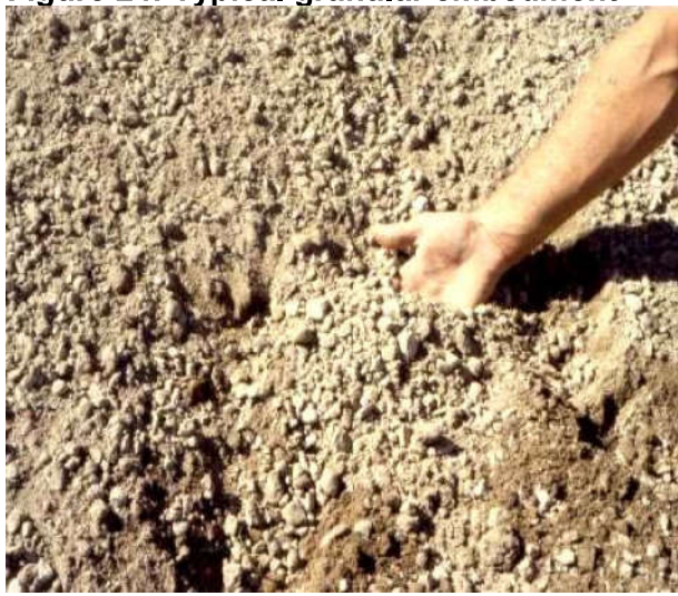
Figure 24: Typical granular embedment
